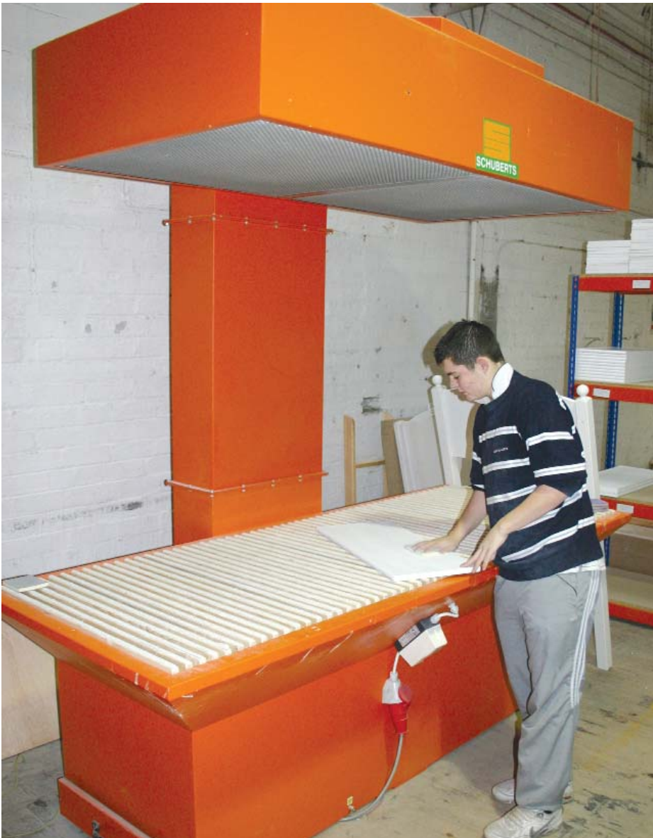
Left: Peter Schubert's unique sanding table sucks dust down through the filters under the table, then returns it as warm air via a second filtration system at the top. Ex stock for under £3k. Also available without recirculation or without filter system.
