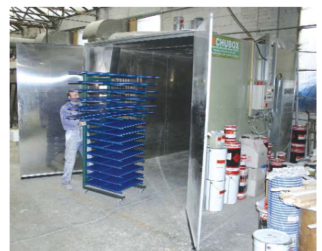
Above: Cresta's Schubox was the first Schubert Technical services supplied. It's a 3-section unit with 2 catalysts which runs on propane.
