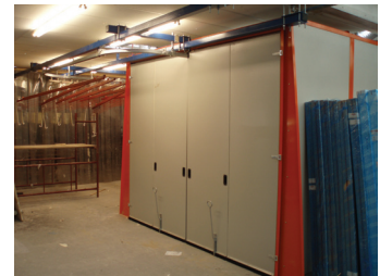
Extra wide 3m Schubox with special bi-fold doors and cut outs for conveyor system
