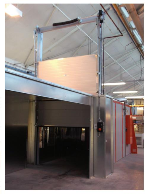
Over a three-day period, Schuberts delivered, installed and commissioned a bespoke flash-off section, Schubox with an automatic door system. The freshly-sprayed pieces are placed into a dedicated flash-off zone, which allows solvent vapour to vent off for 10-15 minutes, before being placed inside the Schubox catalytic IR drying system for a maximum time of 20 minutes.
